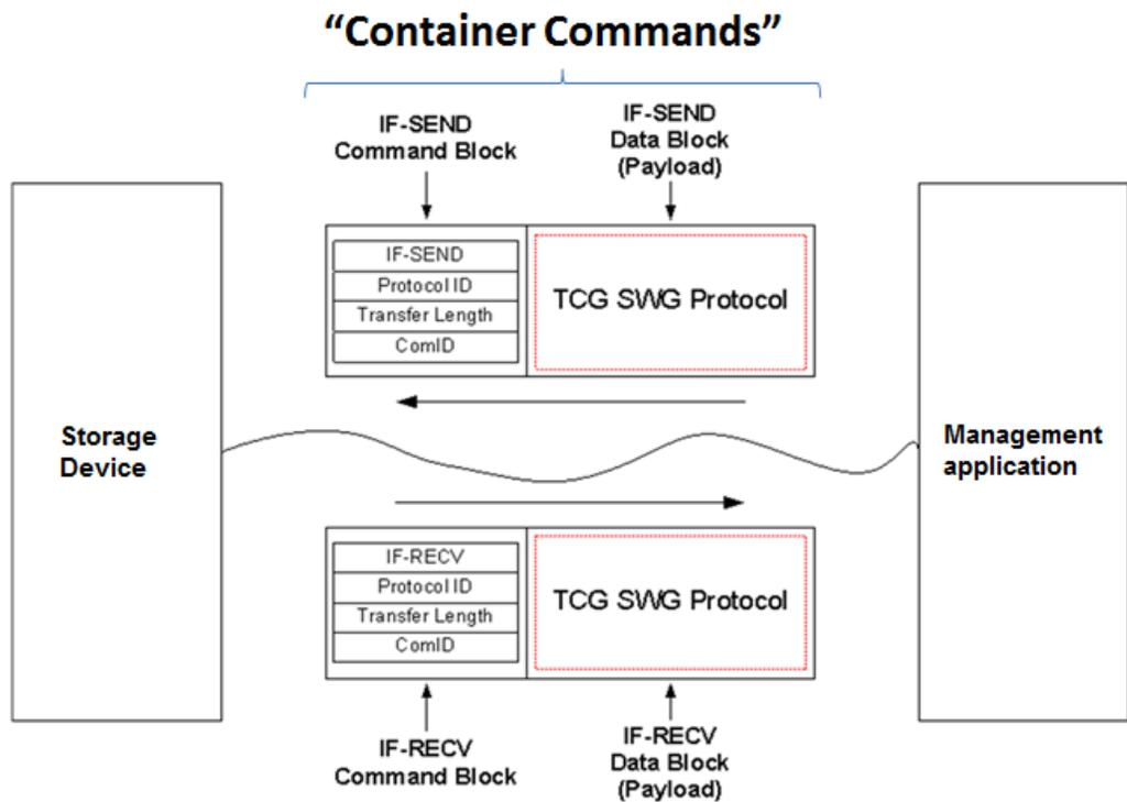
Storage Devices that implement Opal are built to protect the confidentiality of stored user “Data at Rest” (DAR) against unauthorized access once it leaves the owner’s control, when or after the Storage Device has been power cycled.
